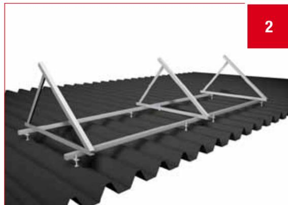
Alternative 2: A sliding block is clicked into the upper WASI 1 rail channel and the elevated mounting is attached with a DIN 912 M8 Allen screw (length depends on the strength of the elevated mounting) that is screwed into the sliding block.
