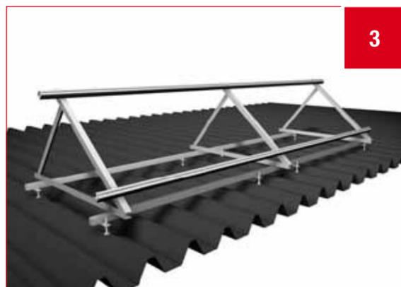
PICTURE 3: Upper attachment: You attach the system units in a similar manner to the adjustable elevated mountings, but without using mounting platelets. A DIN 933 A2/A4 10 x 25 hexagon bolt is pushed into the lower channel of the system units such that the thread sticks out downwards. The thread is pushed through the drill hole on the diagonal branch of the elevated mounting, countered and fastened with a 9345-2-10 locking nut or a 985-2-10 stop nut.
