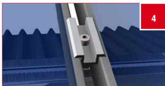
PICTURE 4: Swivel the sliding block into the upper rails and click it in. You twist the middle clamp into the sliding block with the respective screw (depending on the module height). Alternatively, you can attach click-in kit in the upper channel of the rails and screw it tight (tightening torque up to a maximum of 18 Nm depending on module manufacturer.)
