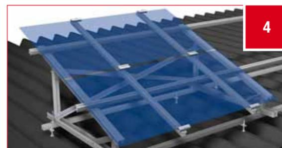
PICTURE 4: Swivel the sliding block into the upper rails and click it in. You now twist the clamp into the sliding block with a DIN 912 A2/A4 M8 x 35 mm screw and screw it tight (tightening torque up to 15 Nm.)
