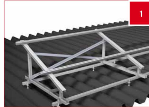
PICTURE 1: Once all of the module units have been mounted to the brackets, you attach the cross-bracings. You can make use of common L-sections (40 x 40 x 3) for this. You must mount them to every closed row once and at least every 12m. You can screw these sections directly onto the rear brackets with drilling screws or attach them with normal standard screws.
