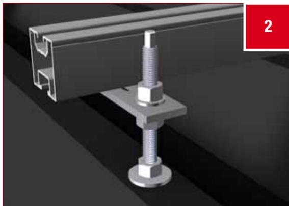
Once you have mounted all of the adapter sheets, the system units are attached to the adapter sheets. For this, thread the hexagon bolts DIN 933 A2/A4 M10 x 25 mm into the respective rails and tightened with the locking edge bolts 9345 A2/A4 M10 to the adapter sheet (tightening torque 9-10 Nm).
