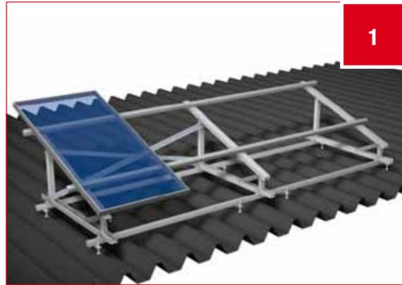
PICTURE 1 & 2: Once all of the module units have been mounted to the brackets, you attach the cross-bracings. You can make use of common L-sections (40 x 40 x 3) for this. You must mount them to every closed row once and at least every 12m. You can screw these sections directly onto the rear brackets with drilling screws or attach them with normal standard screws.
