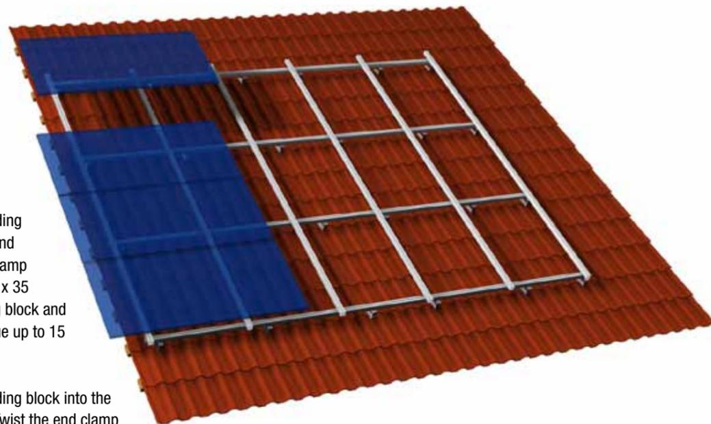
PICTURE 1: Swivel the sliding block into the upper rail and click it in. Twist the end clamp with a DIN 912 A2/A4 M8 x 35 mm screw into the sliding block and tighten it (tightening torque up to 15 Nm.)
