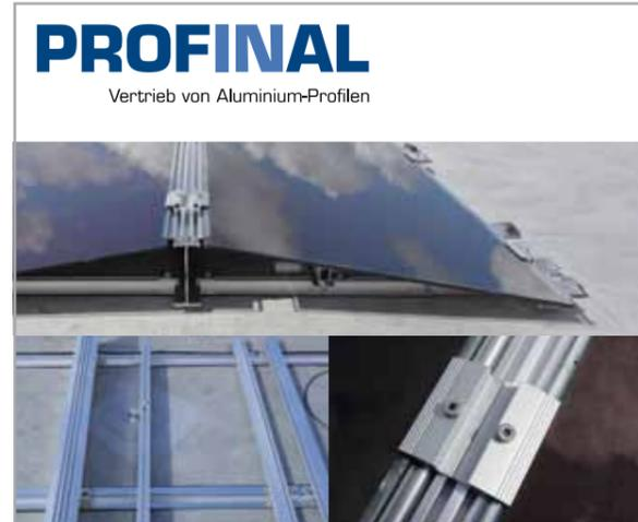
The North Mount System is suitable for frameless solar modules from GS-Solar and First Solar. The simple and versatile mounting system for thin film modules is supplied as a preassembled support structure with integrated screw channels. In addition, stencils help to ensure a custom-fit installation.
