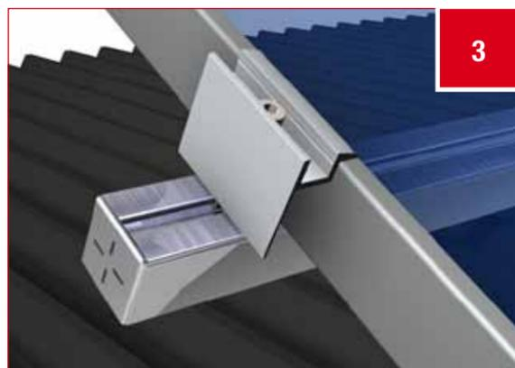
PICTURE 3: To attach the module clamps, swivel the sliding block into the upper rails and click it in. You now turn the end clamp and its respective screw (depending on the module height) into the sliding block. You could alternatively attach the click-in kit in the upper channel of the rails and screw it tight (tightening torque up to a maximum of 18 Nm depending on the module manufacturer). You can add a cover to the rails for personal or appearance reasons.
